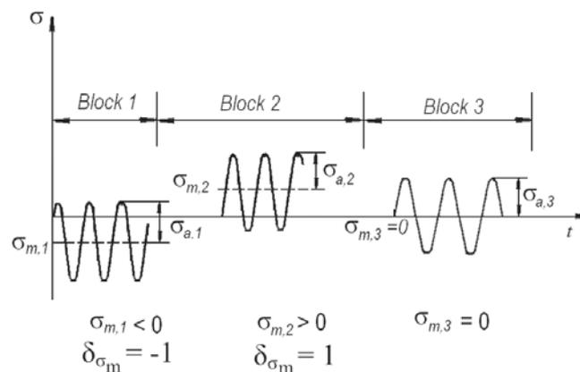
Fig. 4. Three different blocks of cyclic normal stresses.
